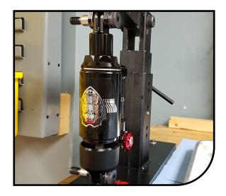
Remove air can, bumper, and spacers (if present). These may remain in the air can, locate and save for later reassembly.
