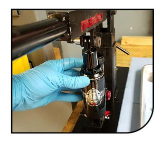
Tighten air can onto shock until the hard stop. Do not tighten past this point.
