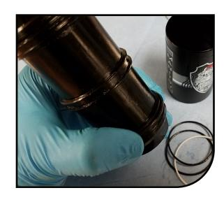
Lightly Grease new O-rings and install into seal glands using a plastic O-ring tool or by hand.
