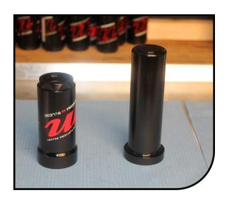
Place the air can onto the seal tool or onto a flat surface.
