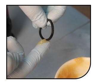
Install the air can quad ring into the lower groove in the air can. Ensure it is not twisted.
