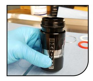
Remove the upper and lower O-rings. (Remove Mid King O-ring if being used.)
